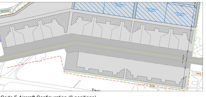
Code F Aircraft Configuration (6 positions) Scale 1:5000
